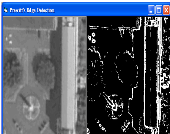
Fig.3 Gray level image and binary edge diagram of TCMT (Source: Google Earth)
