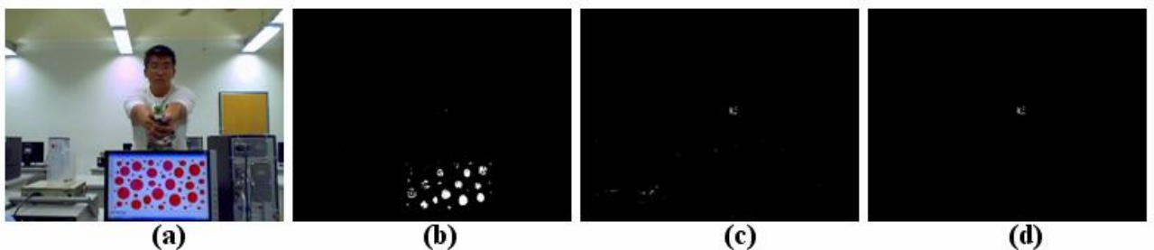
Fig. 3 The background image with more red pixels: (a) Original image; (b) binary Br image of (a); (c) the binary Bg image of (a); (d) the resulting image of TR.
