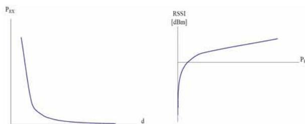
Fig. 4 (a) Received power  $P_{RX}$  versus distance to the transmitter (b) RSSI as quality identifier of the received signal power  $P_{RX}$
