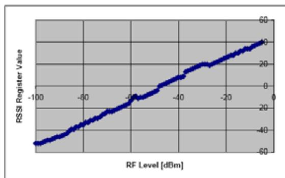
Fig. 2 A contract relation between typical RSSI with input power.
