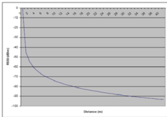
Fig. 3 The relation curve between RSSI with distance.
