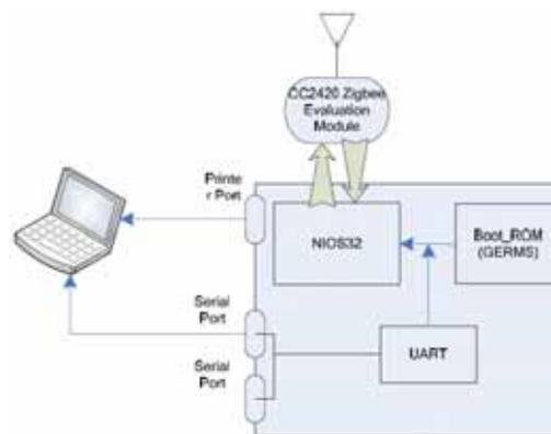
Fig. 5 The hardware framework in SOPC development platform established ZigBee wireless communication device.
