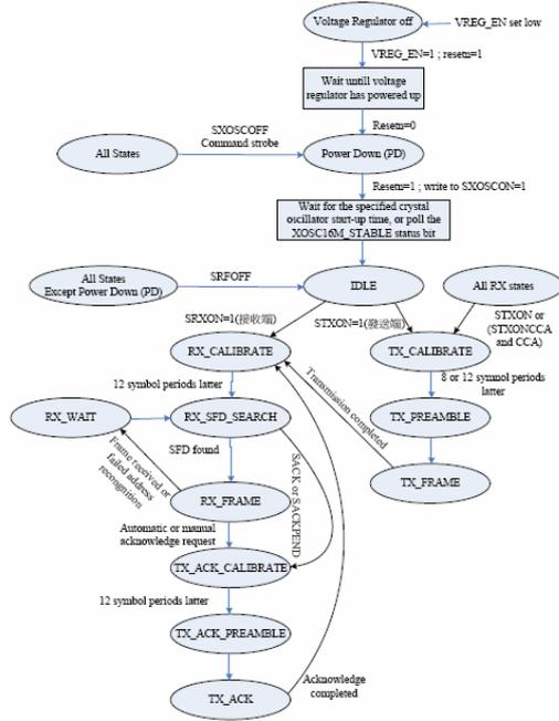
Fig. 6 The Software state control flowchart in SOPC development platform.
