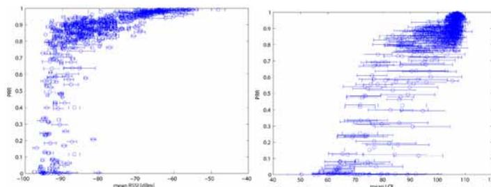
Fig. 10 The RSSI and LQI location engine performances curves
