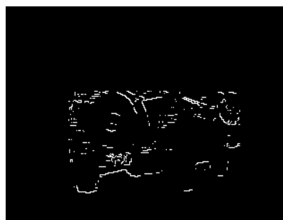
Fig. 11. The residual skeleton image after deleting over- size skeletons
