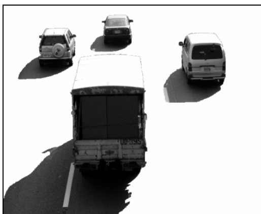
Fig. 5. The moving vehicles apart from the background in the scene are extracted from original image.
