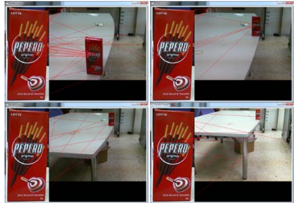
Fig. 6 Difference distance of the object with camera, the effect of SIFT will be affected.
