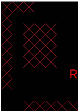
Fig. 9 Probability map, the “R” is mean robot, “X” is mean the obstacle.
