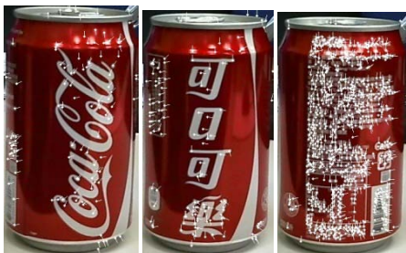
Fig. 8 The SIFT feature points in difference sides of the object Coke can.
