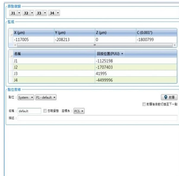
Figure.6-2 Rotation degree of each motor axis
