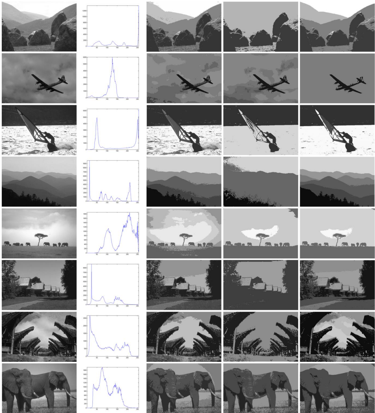
Fig. 12. Thresholding results of the UC Berkeley dataset [14]. The 1st column: original images, from top to bottom, which are UCB-1, UCB-2, UCB-3, UCB-4, UCB-5, UCB-6, UCB-7, and UCB-8, respectively. The 2nd column: histograms corresponding to the input images. The 3rd column: images thresholded by SEZ [3]. The 4th column: images thresholded by FET [1]. The 5th column: images thresholded by the proposed method.
