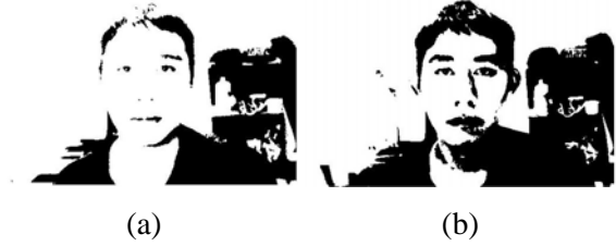
Fig. 4 (a) Binary image when threshold T=60 ; (b) Binary image when threshold T=0 .
